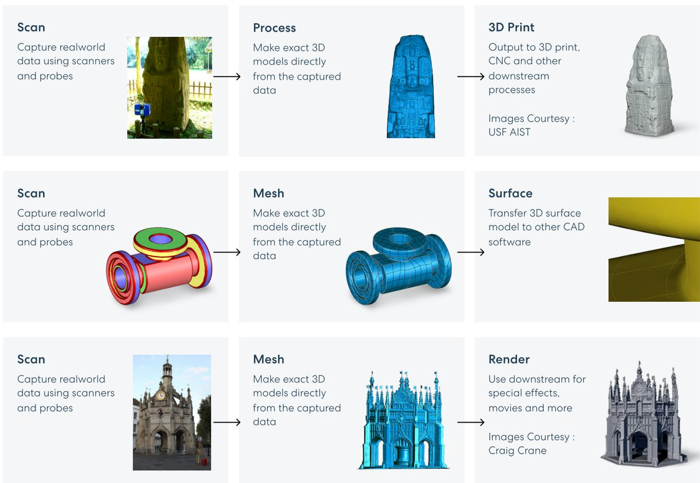
**Geomagic Wrap supports all 3D digitizers, cameras, and scanners in XYZ/ASCII format, and it handles ordered and unordered surface and volume data.**
